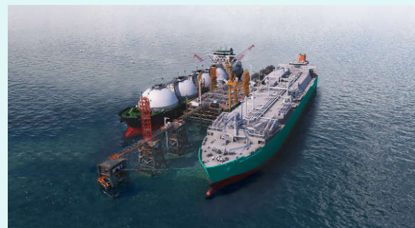
The offshore LNG terminal project is under development by CLP Power and HK Electric (simulated photo).
